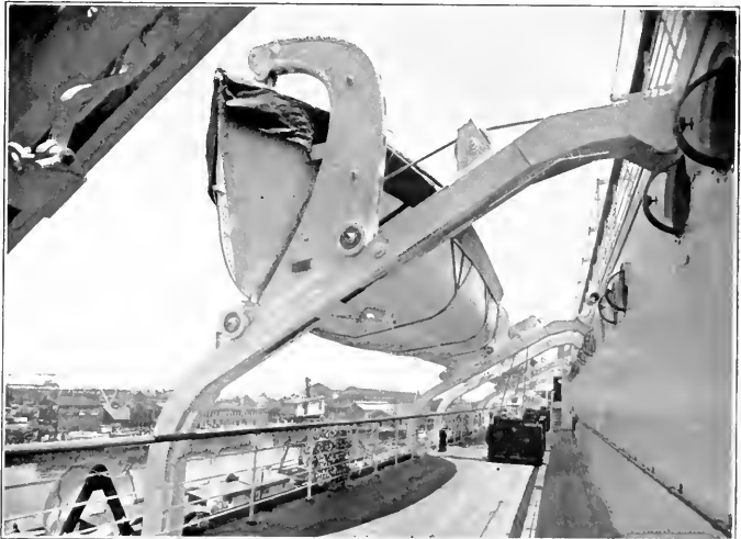
View on the boat deck showing 92-person Welin lifeboats mounted on Welin-MacLachlan gravity type davits equipped with winches for raising the boats.
